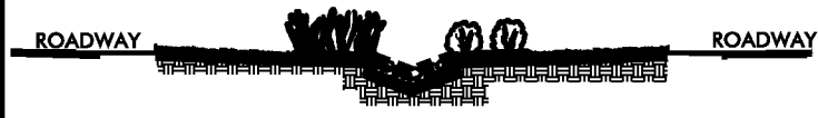
CLASS "A" STONE DITCH LINING DETAIL MIN. 12" DEEP CLASS "A" STONE ON FILTER FABRIC LINER IN DITCH. PLACE STONE FLUSH WITH DITCH GRADE FOR MAXIMUM WATER FLOW.
