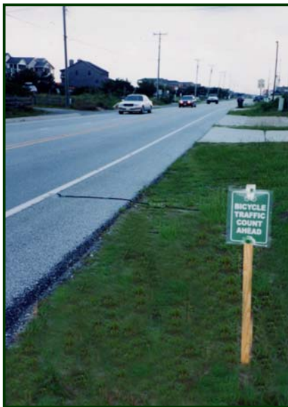
Left: Example of pneumatic tube across a wide paved shoulder. Note the sign alerting cyclists to the counter ahead. Photo courtesy NCDOT Above: A close-up of the sensor itself, which stores the number of counts per hour per day. Photo courtesy ITRE
