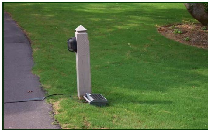
Left: Example of pneumatic tube across a wide paved shoulder. Note the sign alerting cyclists to the counter ahead. Photo courtesy NCDOT Above: A close-up of the sensor itself, which stores the number of counts per hour per day. Photo courtesy ITRE
